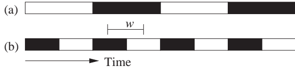
Figure 9: Two voting systems, (a) and (b), with the same availability but different MTTF and MTTR. White boxes on the time scale show when a particular system is up and black boxes show when it is down. The regeneration window is w .
