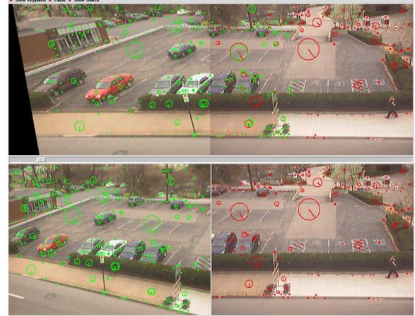
Figure 3. Automatic stitching of multiple camera images for the Parking Space Finder using keypoints. The circles mark PCA-SIFT interest points in the lower two source images. A few closely matching keypoints suffice to generate a transform mapping one image’s coordinates into the other’s and to enable fully automated stitching.
